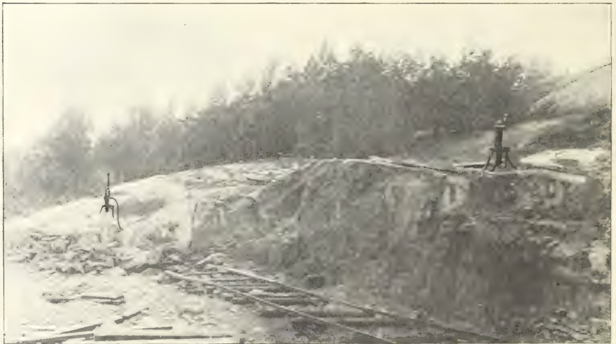
Ledge where stone is obtained, showing two compressed air drills. 500 lbs. of dynamite is required for one day's work
